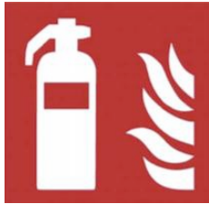
Location fire extinguisher
